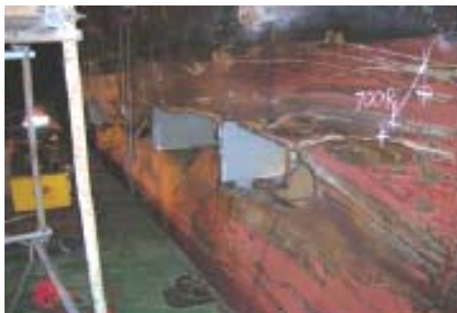
Ribbing Repairs to MV Provider
